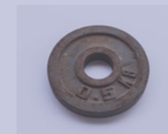
Counterweight It is used to throw tie-rods over the stack. Any object weighting at least 200 g can be used.
